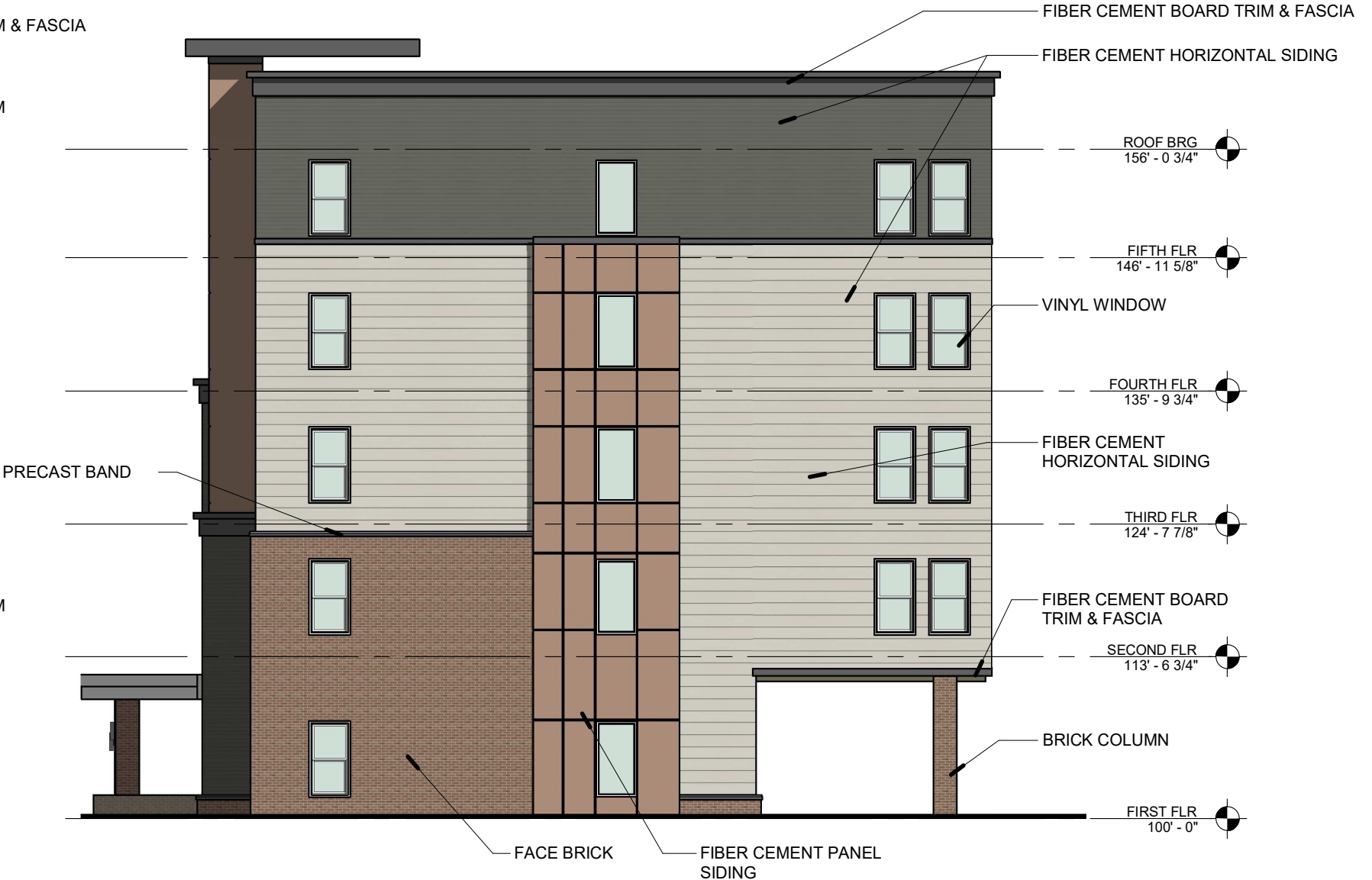
4 WEST ELEVATION PR-4.2 3/32" = 1'-0"
