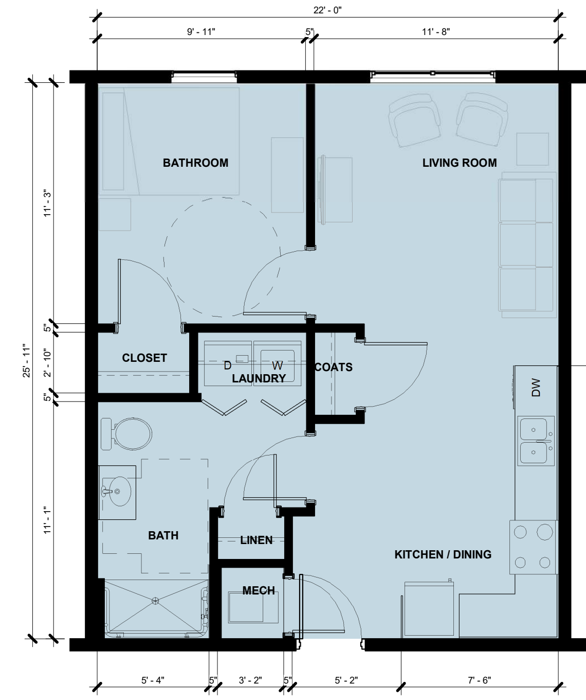
TYPICAL ONE BR UNIT - 1BR-2 - TYPE A / ADAPT. 1/4" = 1'-0" 568 SF NET / 609 SF GROSS
