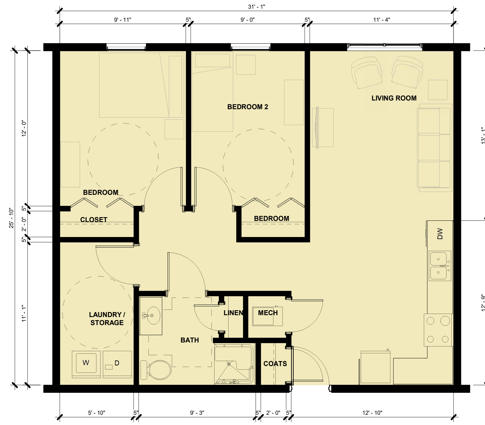
TYPICAL TWO BR UNIT - 2BR-2 - TYPE A / ADAPT. 1/4" = 1'-0" 805 SF NET / 855 SF GROSS
