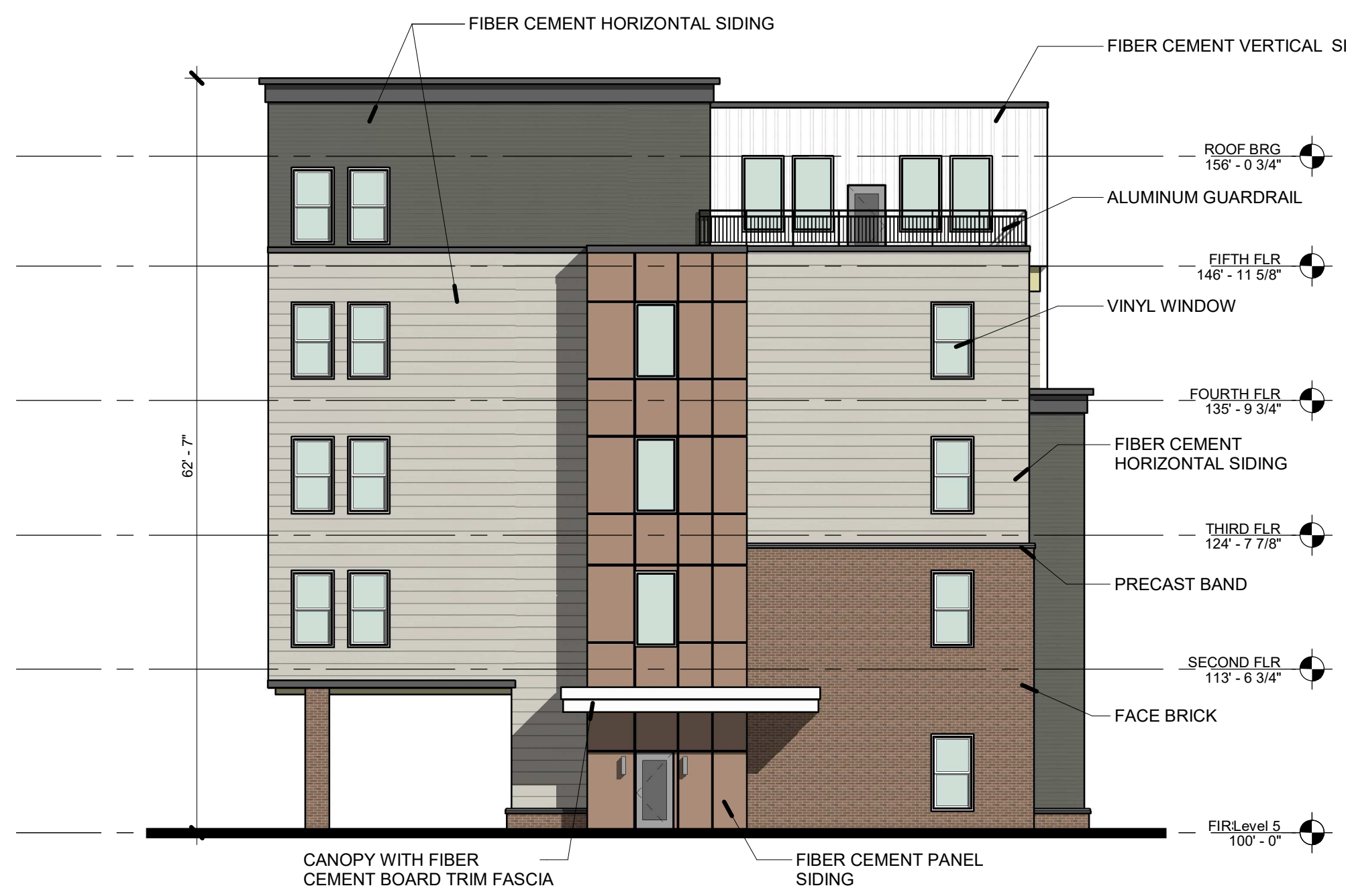
2 EAST ELEVATION PR-4.2 3/32" = 1'-0"
