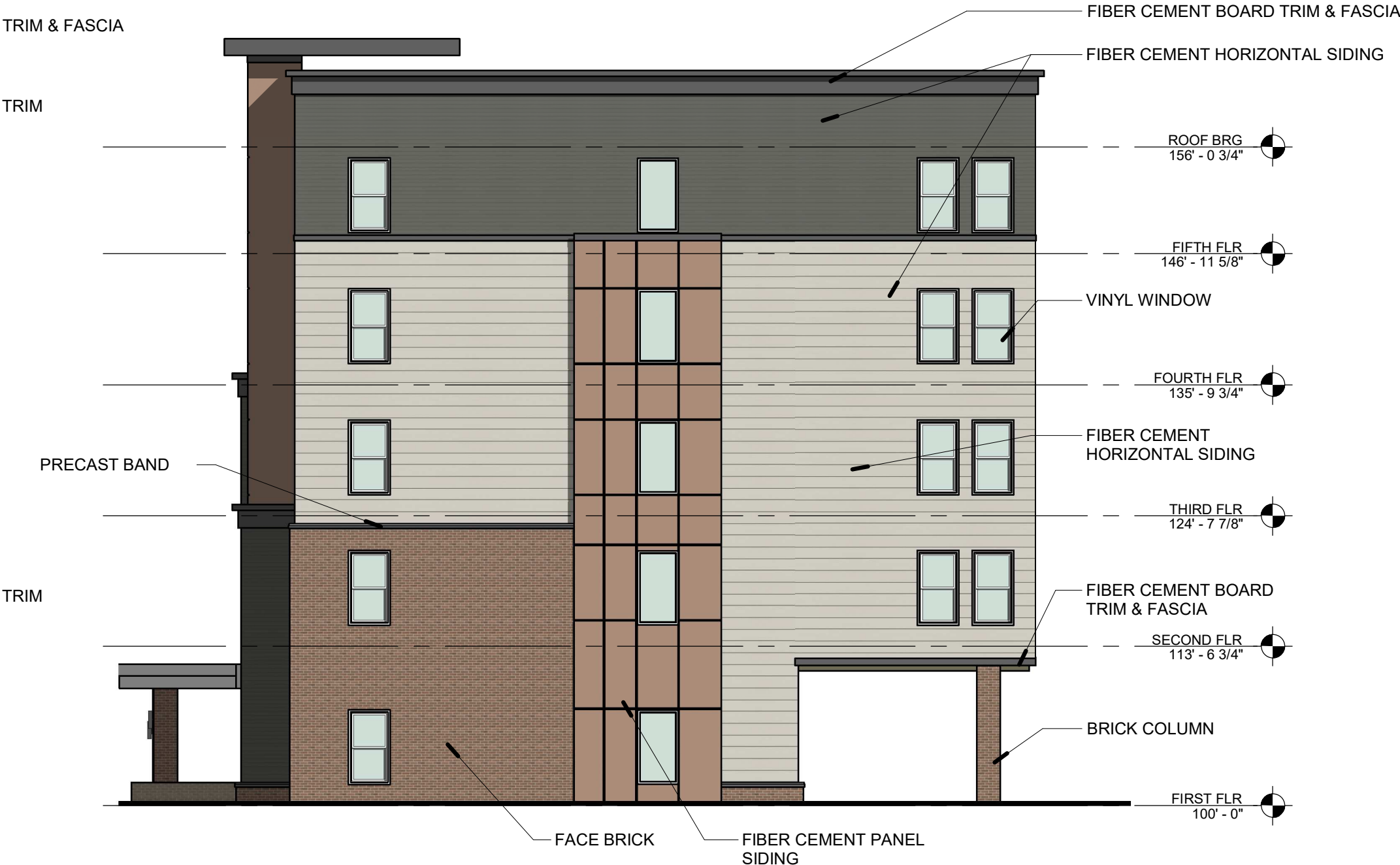
4 WEST ELEVATION PR-4.2 3/32" = 1'-0"
