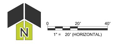
COORDINATES AND BEARINGS ARE BASED UPON THE ILLINOIS STATE PLANE COORDINATE SYSTEM, EAST ZONE (NAD 83), ADJUSTED TO GROUND VALUES, AS ESTABLISHED BY REAL-TIME KINEMATIC (RTK) GLOBAL NAVIGATION SATELLITE SYSTEM (GNSS) UTILIZING GPS OBSERVATIONS. UNITS ARE IN INTERNATIONAL FEET.
