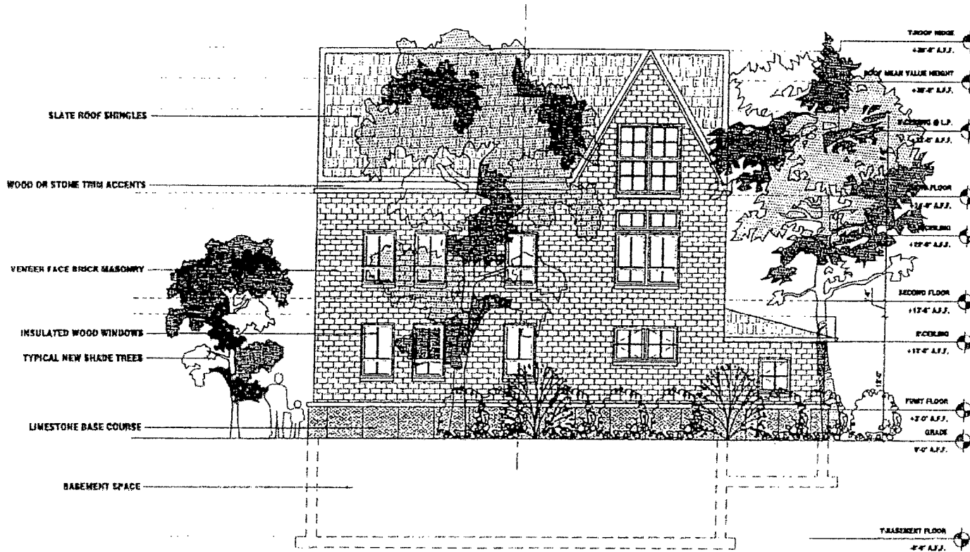
2 SIDE ELEVATION - A HOUSE TYPE 01 - 40'-0" x 46'-0"
