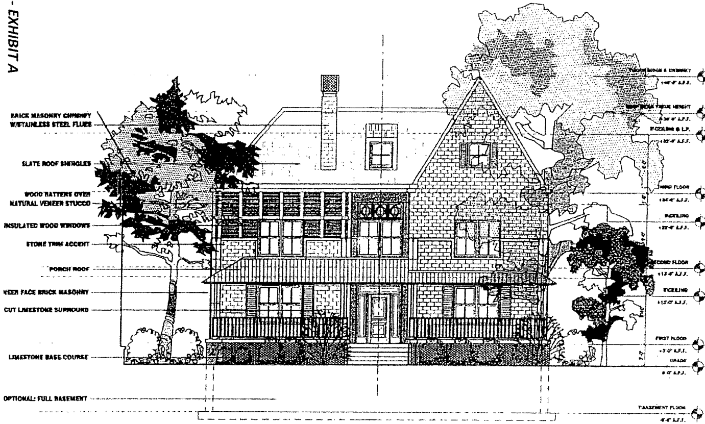
1 FRONT STREET ELEVATION HOUSE TYPE 08 - 40'-0" x 46'-0" NOMINAL
