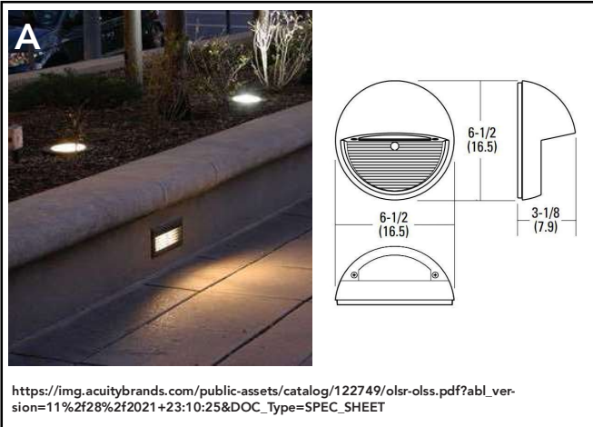
Level 10 (Amenity Deck) Code required step lighting for illuminated pathways - Located at raised planters
