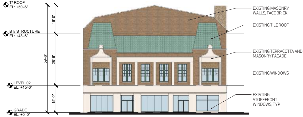
EAST ELEVATION - EXISTING
