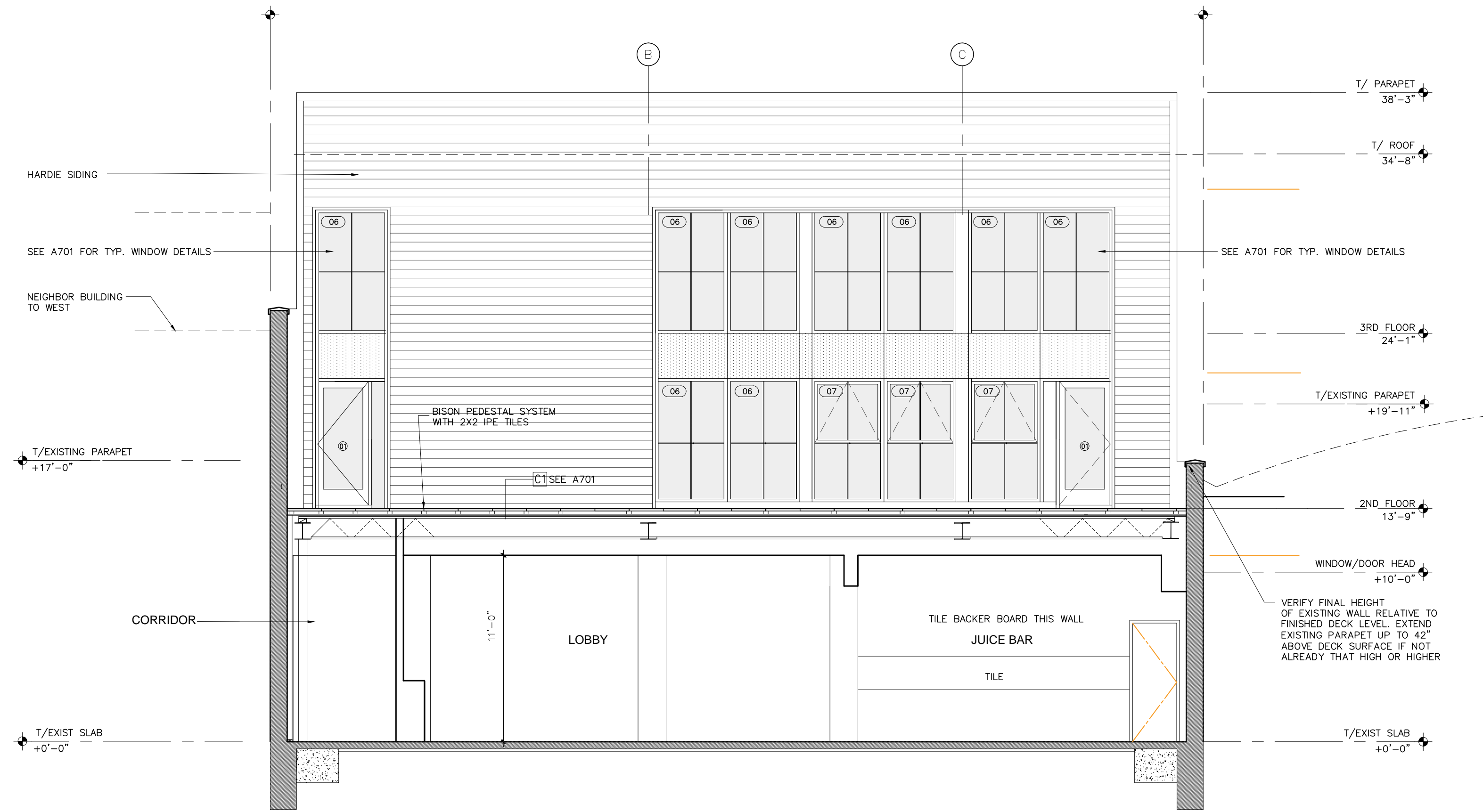
1 BUILDING SECTION @ SOUTH SECTION (FLAT ROOF) 3/16"=1'-0"
