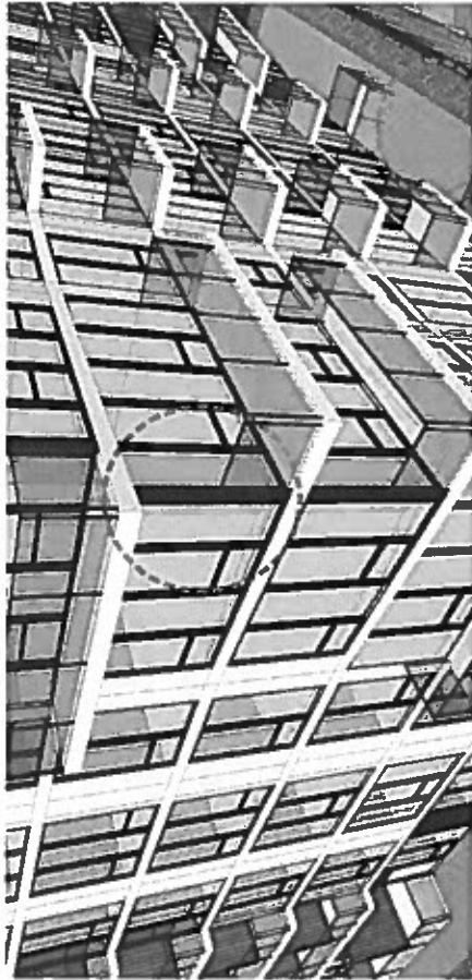
Glazing at building corners will incorporate metal mullions Green roof not to contain taller trees nor shrubs which correlate with more bird collisions (credit: ABC Bird-Friendly Building Design)
