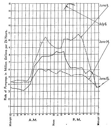
of 14,775,300 gallons per day was held for four hours with a rate maintained over a 5-minute period of 15,800,000 gallons per day, or corrected for slip, of 14,400,000 gallons per day.
