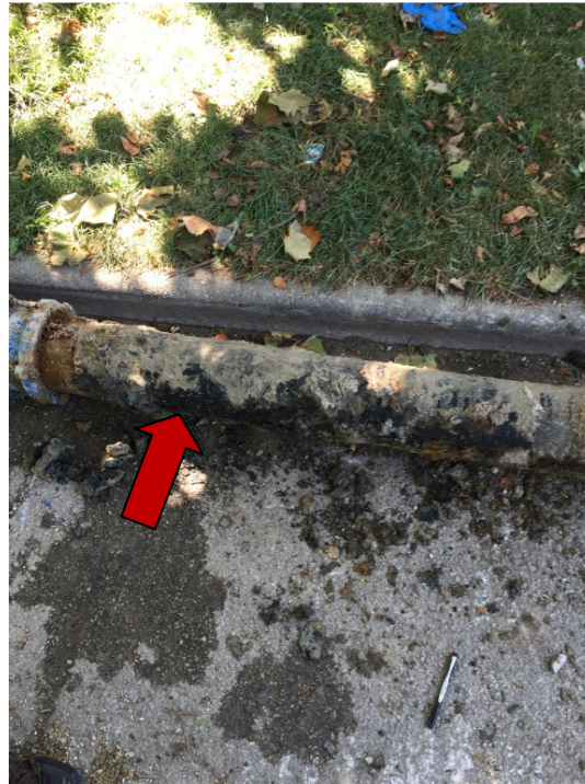
Photo 56: Sample “Exterior Pipe Crust A 78+10/7” was collected on 8/19/15 at 11:20 from a depth of 7 feet. Sample is associated with an 8-inch-diameter, E-W water main on Kirk Street near intersection with Dodge. Sample consists of dark, clayey crust scraped from the exterior of the main (see red arrow). Photo facing south-southeast. By Kramer.
